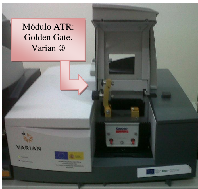
Fig. 3: FTIR: Varian 670-IR. FT-IR Spectrometer. Varian ®.
