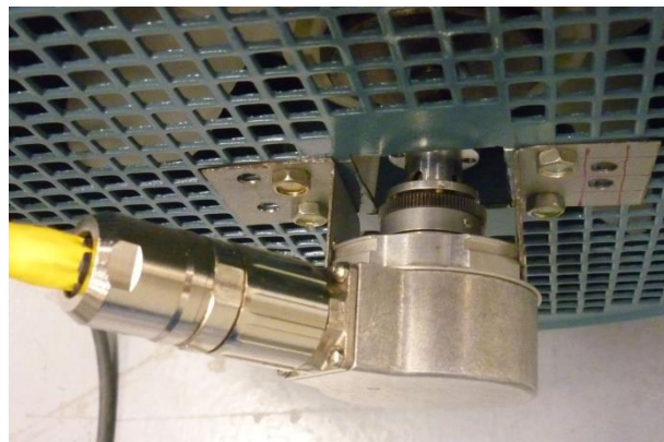
Fig. 29 Encoder attached to the shaft of the machine
