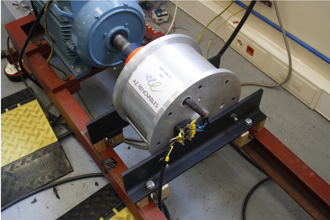
Figure A-3: Generator built by 'AZ Renewables'.
