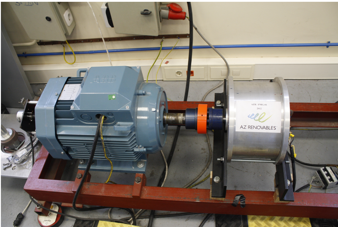
Figure A-4: Photo of the Generator coupled to a induction machine (wind turbine simulator).
