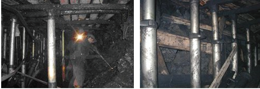
FIGURE 1: Mining labour supported by individual hydraulic props.
