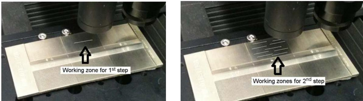
Figure 2. Roughness gauge on 1<sup>st</sup> step measurement (left) and 2<sup>nd</sup> iterations sampling (right)
