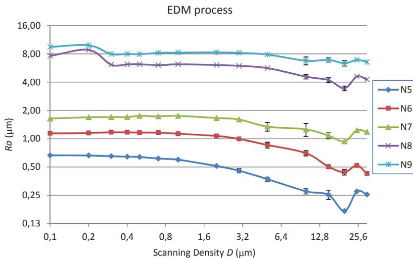
Figure 4. Measured values of Ra for different scanning density measurements over the EDM roughness gauge
