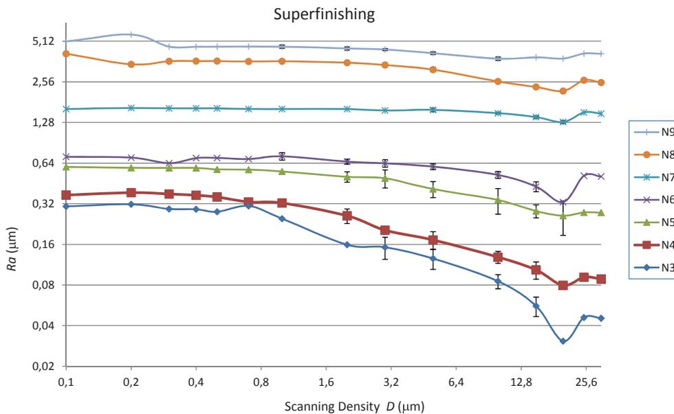
Figure 5. Measured values of Ra for different scanning density measurements over the Superfinishing (N9 to N6) and Honing (N5 to N3) roughness gauges
