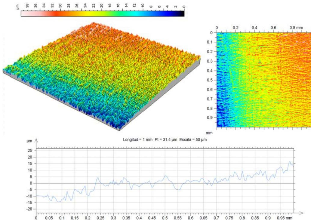
Figure 3. Chromatic 3D map and extracted 2D profile obtained from “turning rugotest” gauge
