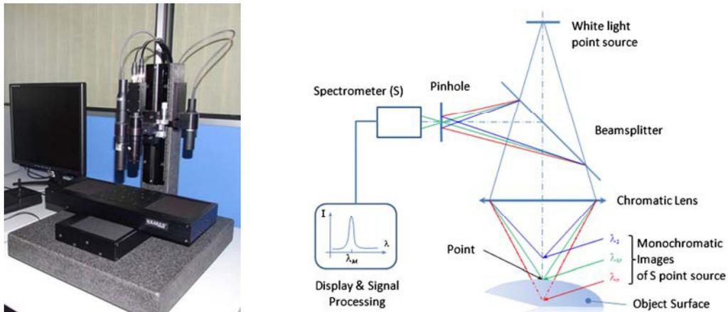
Figure 1. Image and principle of measurement of the Solaris Viking profilometer. Source: Stil S.A., Aix-en-Provence, France.
