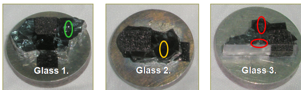
Figure 5.4: Selected glass samples for LA-ICP-MS analyses. Local defects are marked with a circle.
