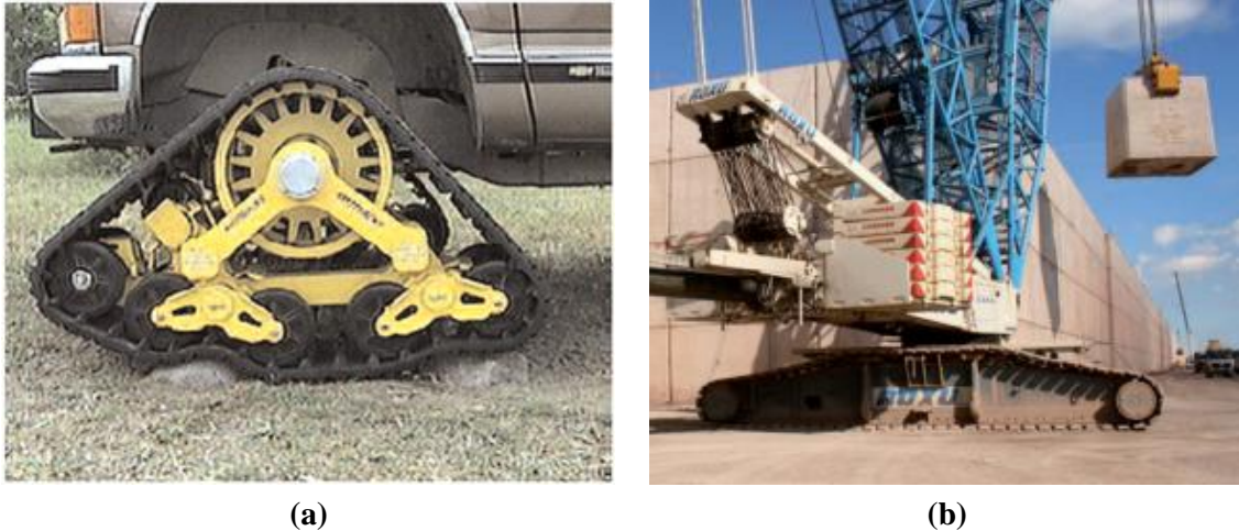
Figure 9. Track crawlers: (a) adjusted to irregular surfaces; (b) track crawler as support of heavy cranes.
