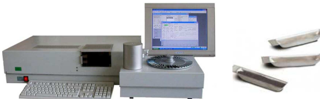
Figure 7: Mercury analyzer AMA-254 and nickel platform/boat
