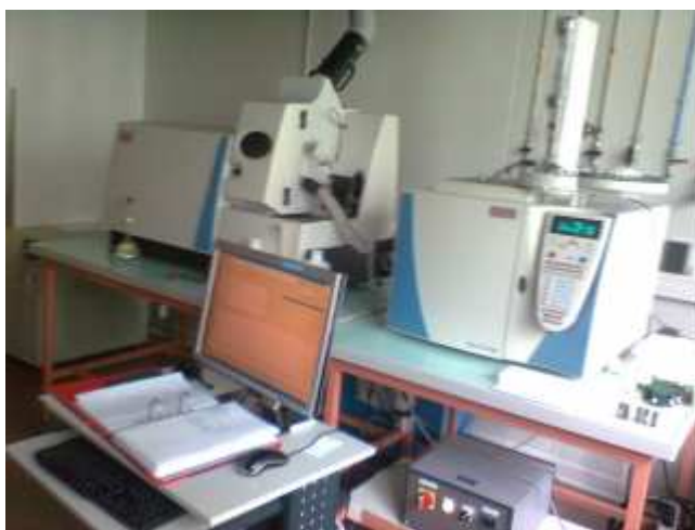
Figure 11: GC-ICPMS used for Hg Speciation analyses at LCABIE
