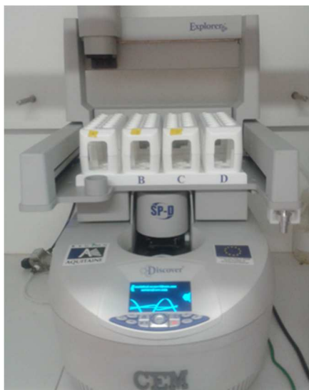
Figure 9: CEM Microwave (Discover SP-D) and CEM Pyrex vessels
