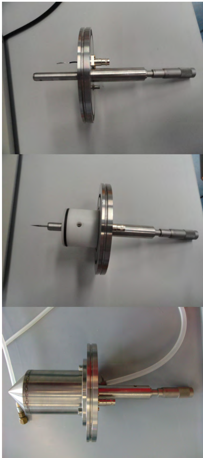
Figure A.o.18: Picture of the corona needle and chamber for ion generation.
