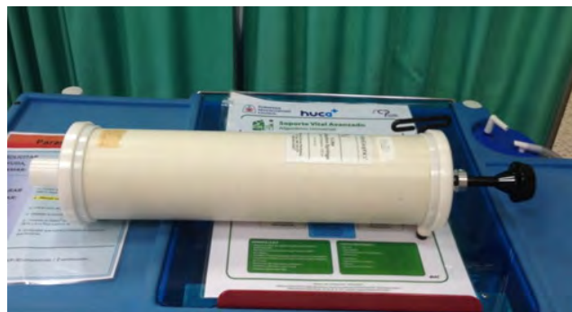
Figure 4.2: Syringe with a volume of 3 L employed for calibrating the spirometer.
