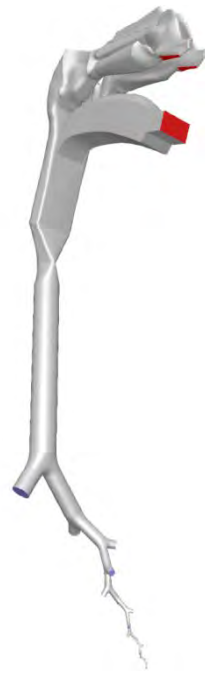
Figure 3.15: Complete tested model, comprising the nose, mouth, pharyngeal region and lower airways, with a single path fully developed up to generation 16.
