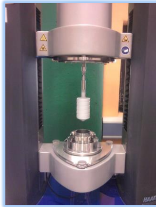
Fig 7.2-2. Haake Mars III rheometer with the Searle system.
