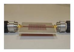
(a) Photo of the suspended microstrip measurement setup.
