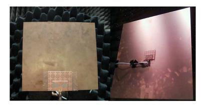
Figure 2.71: Measurement setup in anechoic chamber for Bow-tie-AMC at (Left) the edge and (Right) centered on a metallic plate.
