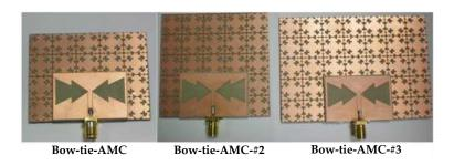
Figure 2.67: Different AMC unit-cells arrangements combined with the double bow-tie antenna: (Left to right) Bow-tie-AMC, Bow-tie-AMC-#2 and Bow-tie-AMC-#3.
