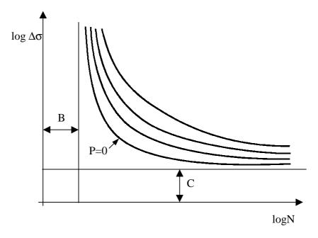
Figure 1: S-N field with percentiles curves in the fatigue model of Castillo et al. [1].
