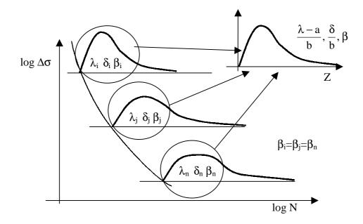
**Figure 2:** S-N field with pdfs of log N at different stress ranges and corresponding pdf of the normalized lifetime, Z.
