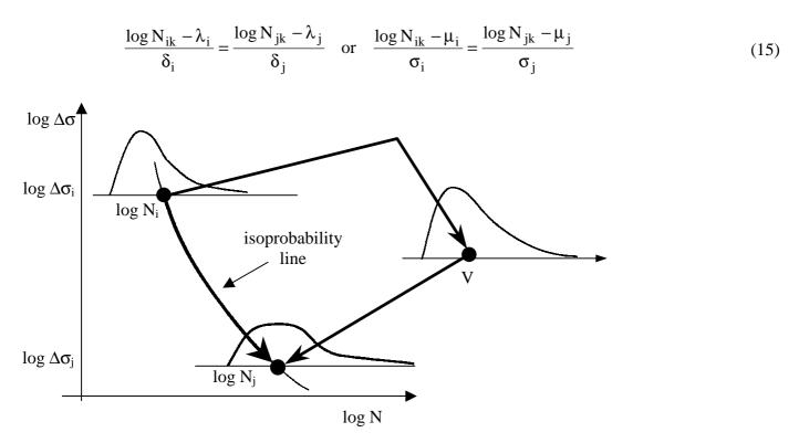
Figure 4: Conversion process with variable V.
