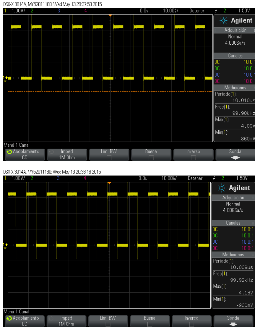
Figure 45, the PWM signals generated on the edge connector to test the configuration of the FPGA PCB.
