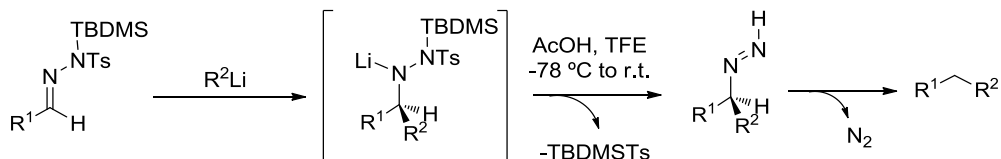
Scheme I.18. Reductive coupling between N -silylated hydrazones and organolithium compounds.
