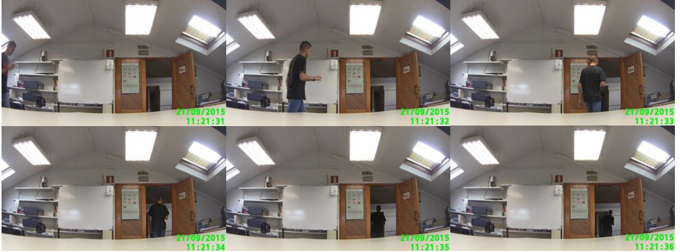
Figure 6 Example of sequence of the pictures that the Canon IP Camera send when detects movement
