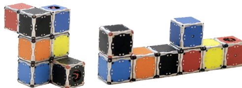
Figure 1.4: A number of cube robots (called M-blocks at Massachusetts Institute of Technology (MIT)) making two different structures. These M-blocks stick together with the help of magnets placed in their corners. [8]
