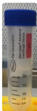
Figura 11. Columnas Macrosep® Advance Centrifugal Device.
