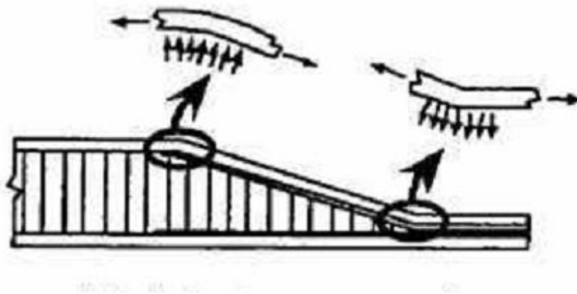
Figure 12.5.- Plane stress in areas of change direction of the bag face
