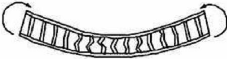
Figure 12.4.- Rupture by bending of the core
