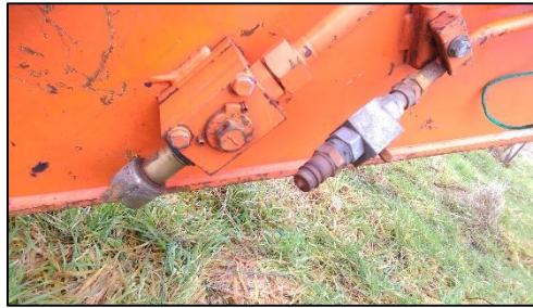
Figure 26: Auxiliary flow outputs on excavator dipper.
