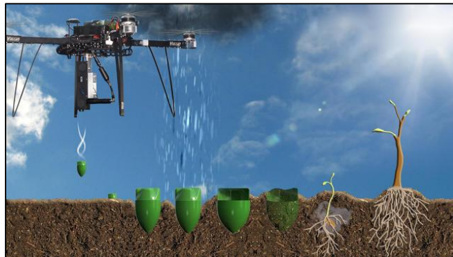
Figure 17: Illustration of tree planting drone showing seedlings being dropped in caplets to the ground [18].
