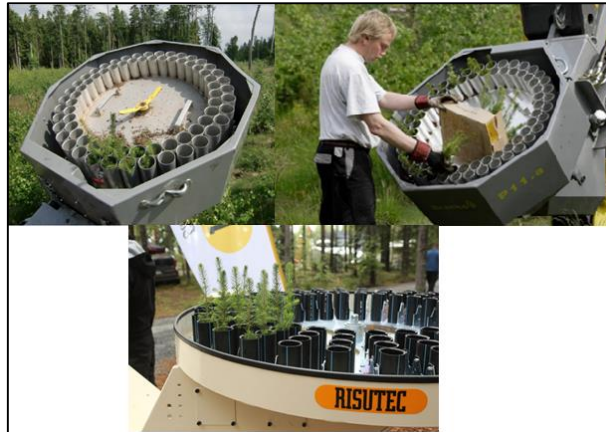
Figure 48: Rotary Carousels: (a) Bracke P11.a [10] (b) Operator manually loading Bracke P11.a carousel [10] (c) Risutec carousel [12].
