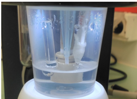
Image 2. Set up of the electrochemical cell.
