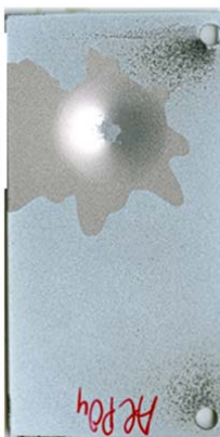
Fig. 46 ATFI composition applied onto SOLFER® steel
