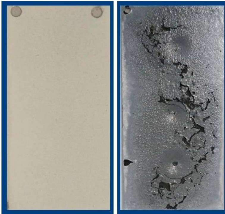
Fig. 8 White top coat applied onto I8 composition the left and white coat applied onto J7 (Solgel) at the right T: 710°C t: 4'
