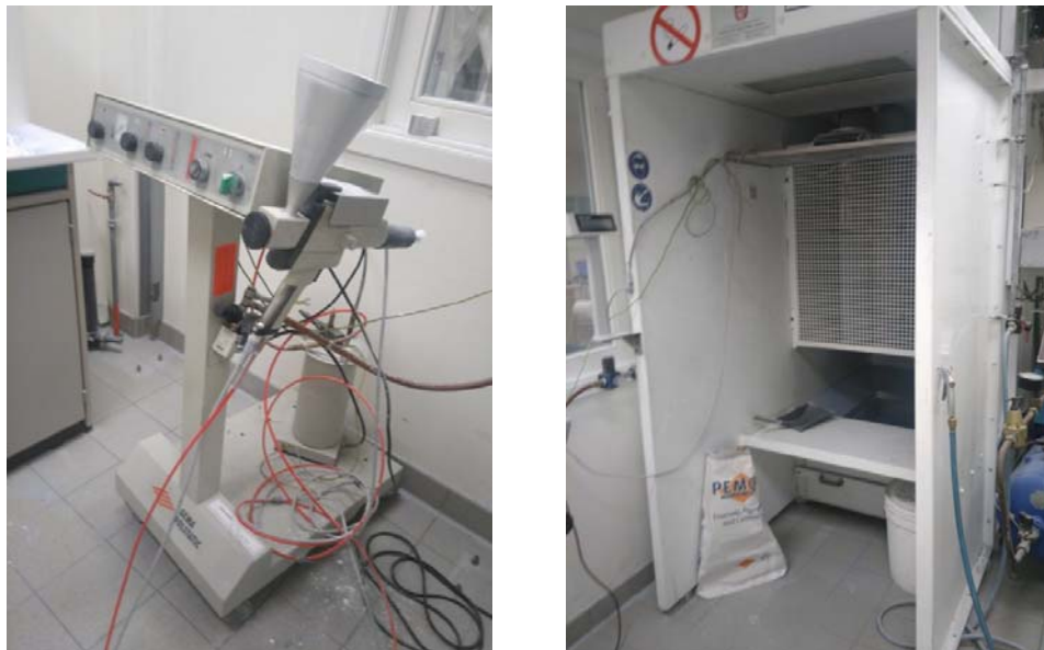
Fig. 20 Left: Electrostatic gun "GEMA VOLSTATIC" and right: extractor to trap the powder
