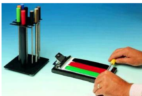
Fig. 16 Hand bar-coating technique
