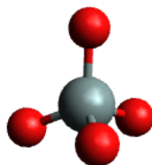
Figura 1. Tetraedro de \text{TO}_4 ( T = \text{Si}/\text{Al} )
