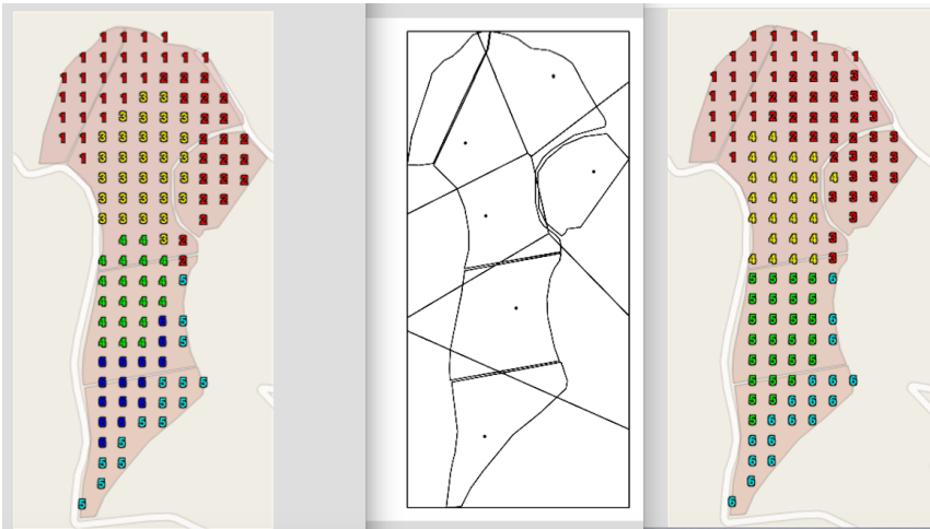
Figure 6.9: The clustering delimitation of Parcel 3 for 6 MZ considering the band B10 (left) and the band 11 (right) has a spatial distribution similar to the one obtained with the Voronoi tessellation (middle)
