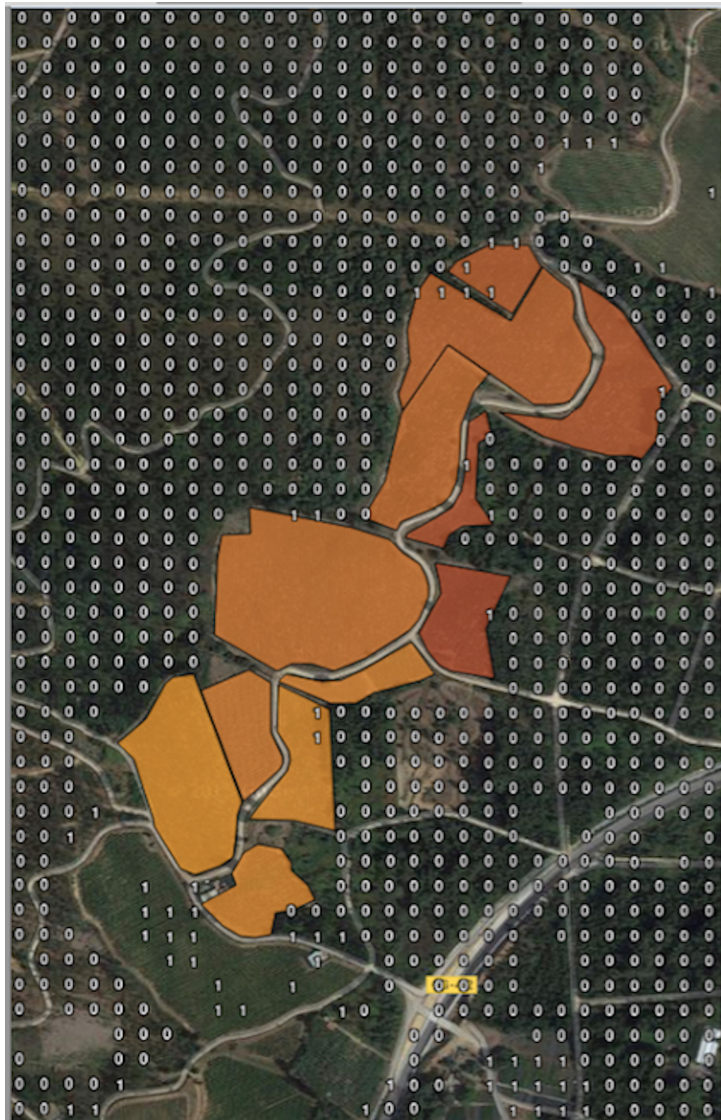
Figure 5.7: Mapping cultivable land cluster for the land parcel 2 with the Band 5 (NIR). The zeroes represent the land correctly classified as non-cultivable. The ones represent the the land incorrectly classified as non-cultivable. The zones without numbers belong to the cultivable-land cluster.
