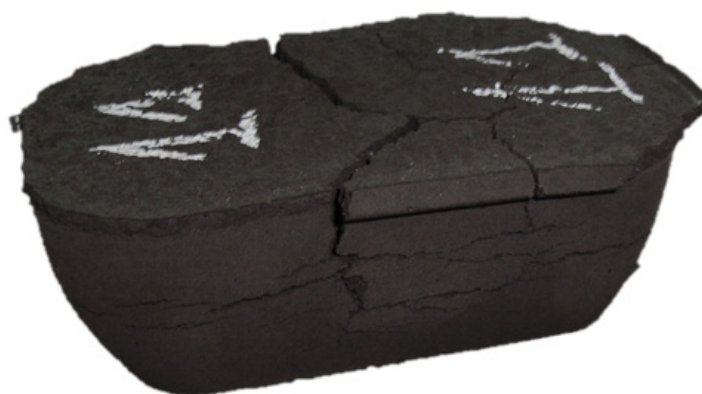
Figure 1. Sample showing cracks (5% Portland cement).
