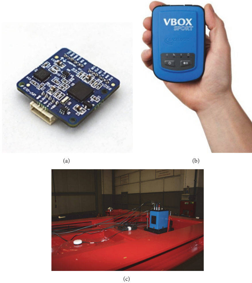
FIGURE 7: (a) Low-cost IMU [6]; (b) GPS VBOX Sport [7]; (c) vehicle sensing with high-accuracy IMU (ADMA-G-EntryLevel, GeneSys) of the validation system.
