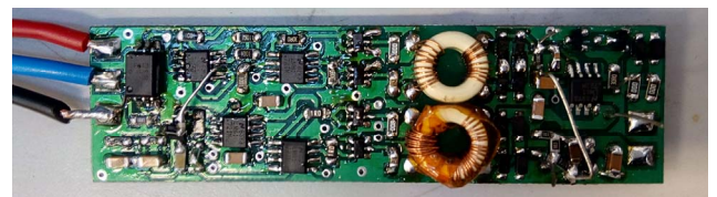
Fig. 8: Prototype of the gate driver (23.9x86.6 mm)
