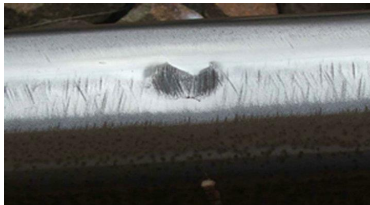
Figure 5. Squat defects in railway [23]
