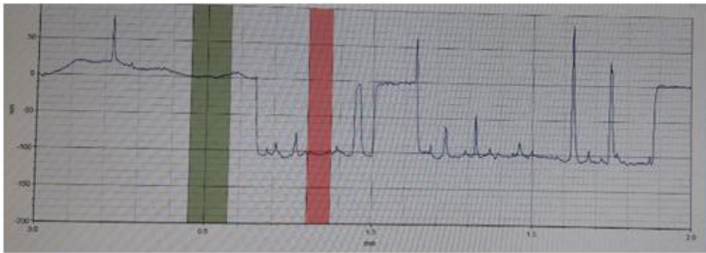
Figure 102 Measured step height profile of a film.
