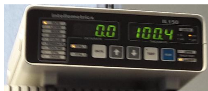
Figure 62 Monitor for controlling the film thickness.
