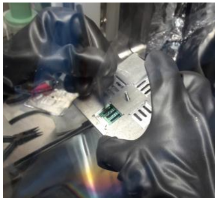
Figure 61 Shadow mask where the active layer is placed.
