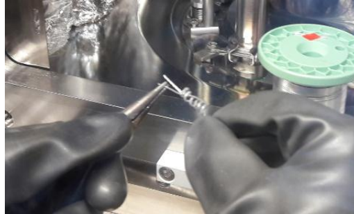
Figure 60 Aluminium wire hang on the filament in the deposition chamber.
