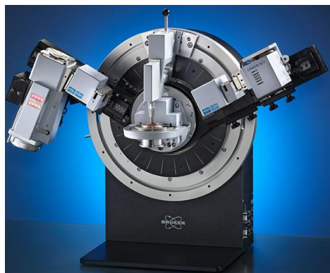
Figure 70 D8 advance with DAVINCI with LYNXEYE detector.
