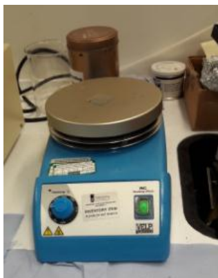
Figure 58 Heating plate for drying the PEDOT. PSS.
