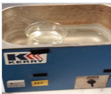
Figure 56 Ultrasonic cleaning tank used to clean the glass substrate.
