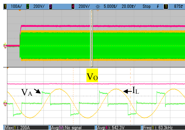
Figure 17. Evolution of voltage V_A [200V/div] and current I_L [100 A/div] in the traditional LCC converter with a load R_O = 586 \Omega , P_O = 500 \text{ W} , V_i = 300 \text{ V} (Fluoroscopy operation).
