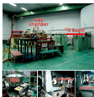
Figure 2. Experimental set-up of the ^{12}\text{C} -rutherford backscattering spectrometry ( ^{12}\text{C} -RBS) measurements.
