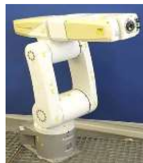
Figure 2. Robot II to be modelled: 6 DOF articulated-arm robot (Mitsubishi RV-3AL).
