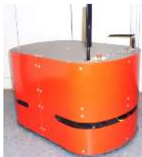
Figure 1. Robot I to be modelled: Autonomous mobile platform (MetraLabs X3).
