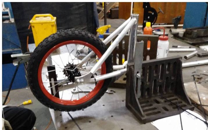
Figure 34: Rig Set-Up for Back Triangle Assembly
