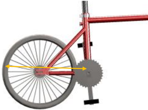
Figure 16: Rear Triangle Showing Limiting Dimension
