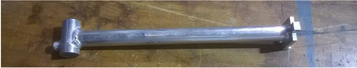
Figure 32: Rotating Tube (Left) Welded to Top Tube & Hinge (Right)
