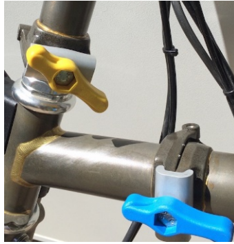
Figure 7: Brompton Handlebar & Top Tube Hinge Mechanism 14
