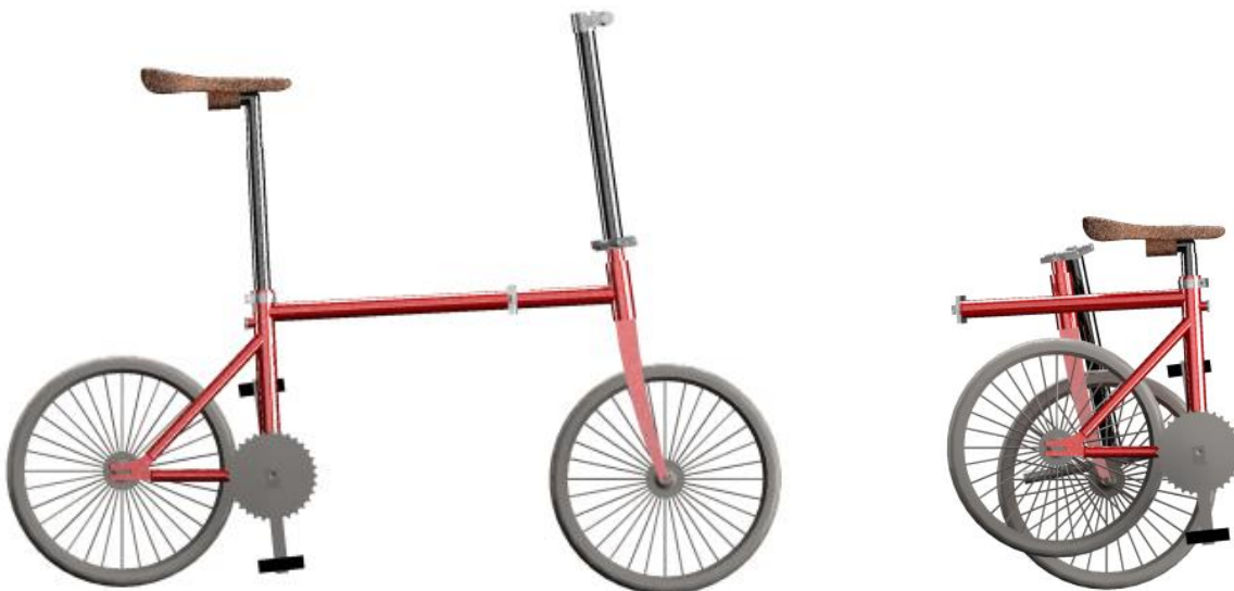
Figure 31: Final Folding Bicycle Design Rendering Unfolded & Folded
