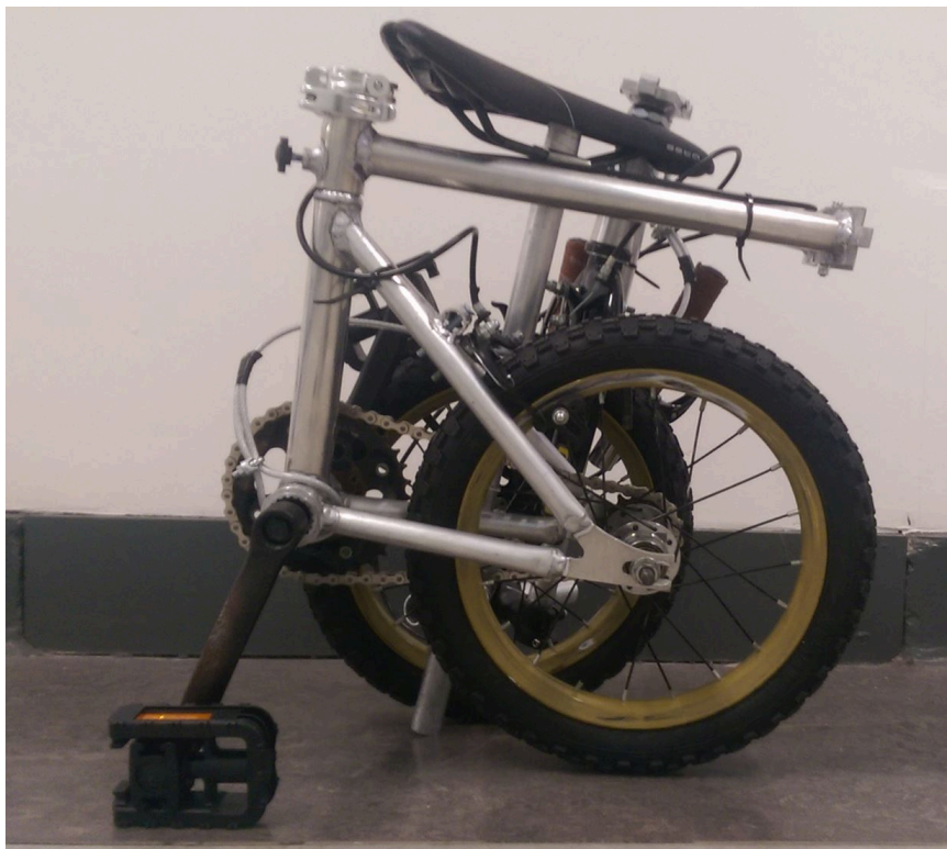
Figure 39: Final Folding Position
