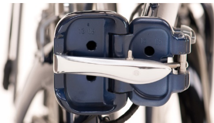
Figure 8: Bickerton Hinge Mechanism 15
