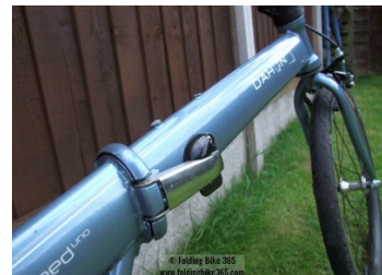
Figure 9: Dahon Hinge Mechanism 16
