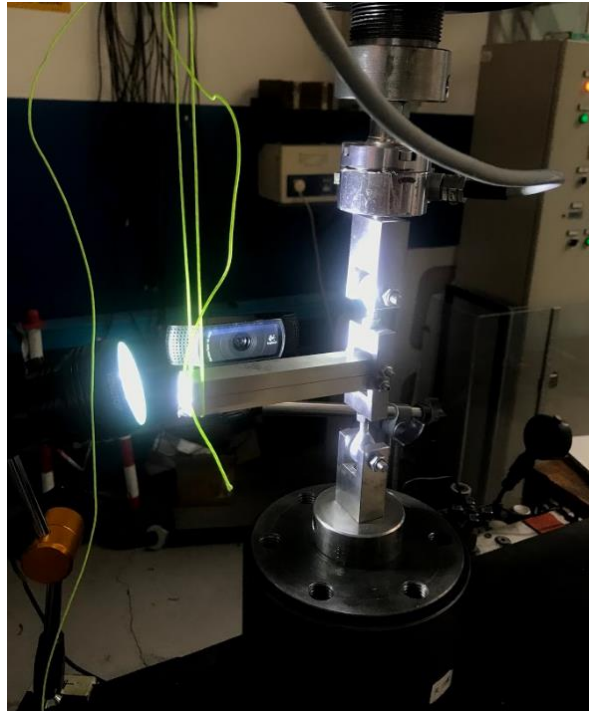
Picture 4-34 DCB test machine with specimen
