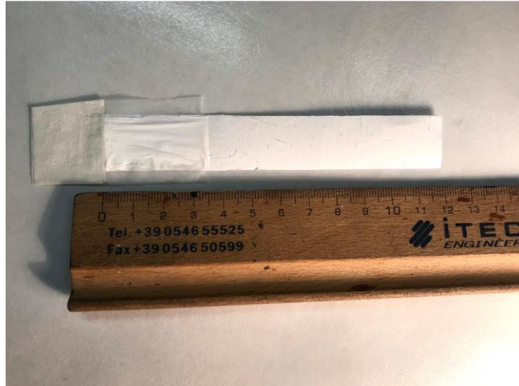
Picture 4-24 Teflon placed inside the nanofiber mat
