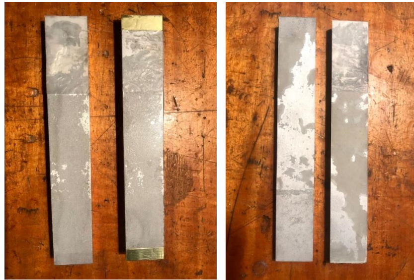
Picture 5-2 Fracture surface of type 2 specimens. Left, virgin. Right, reinforced.
