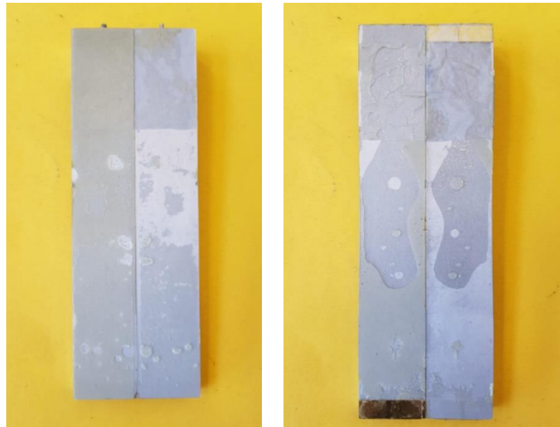
Picture 5-6 Fracture surfaces of batch 4. Left, reinforced specimen. Right, virgin specimen
