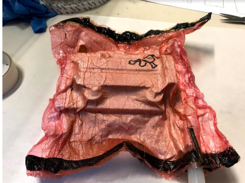
Picture 4-27 Second support inside the vacuum bag
