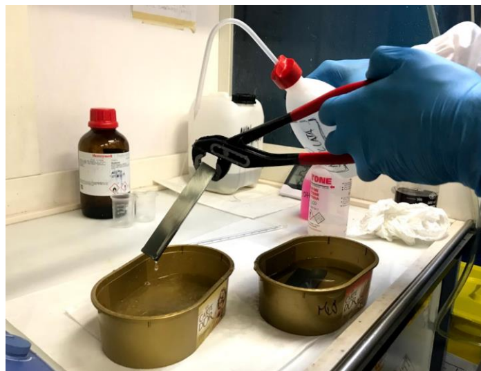
Picture 4-14 Caustic soda solution process
