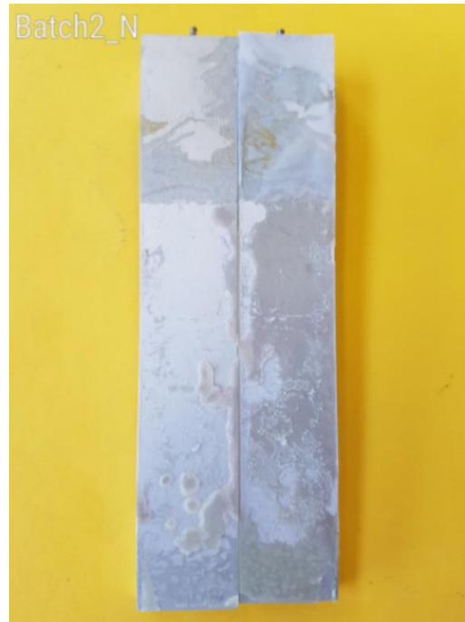
Picture 5-5 Fracture surface of batch 2 nano-reinforced
