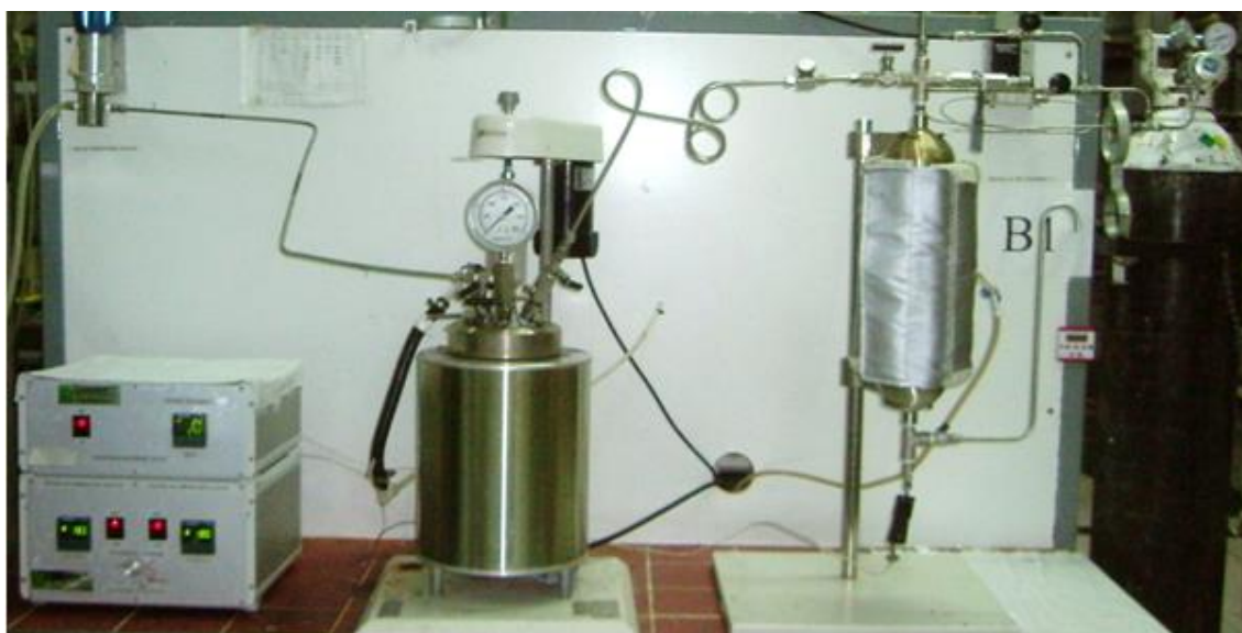
Figure 3.3. Experimental setup used in the thermal hydrolysis and wet oxidation experiments.
