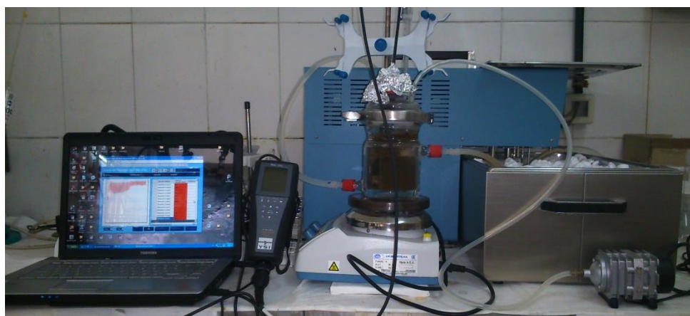
Figure 3.6. Experimental setup used to analyse RBCOD of samples.
