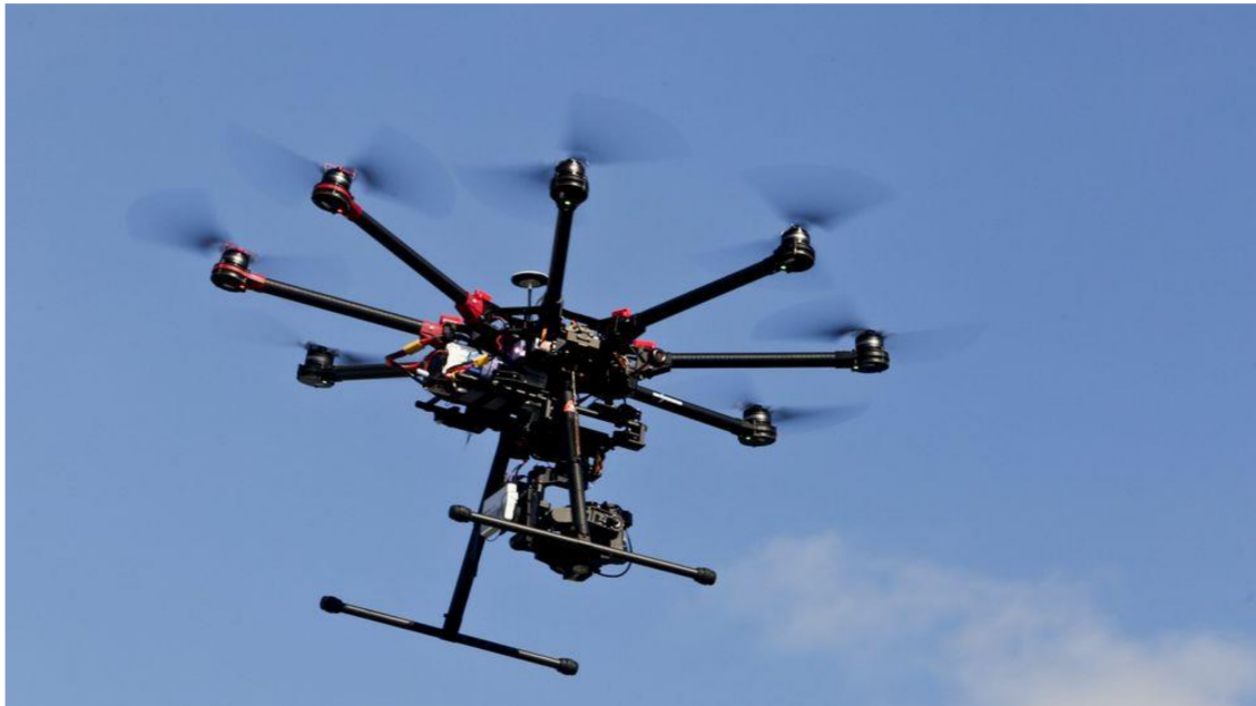
Figure 1. Drone for surveillance missions equipped with camera, GPS, and TV emitter.
