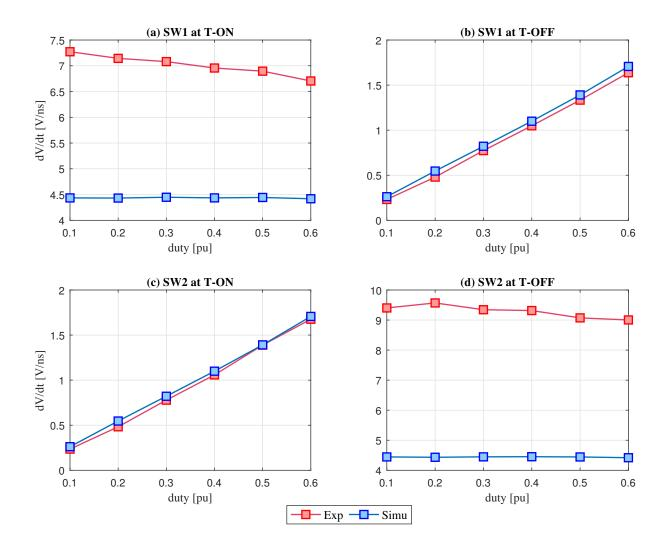
Figure 4-19: Drain-to-source  $(V_{DS}) dV/dt$  in [V/ns] produced in switch 1 (SW1) and switch 2 (SW2), at turn-on and turn-off events for  $V_{in} = 50V$  at different duty-cles: (a) SW1 and turn-on; (b) SW1 and turn-off; (c) SW2 and turn-on; (d) SW2 and turnoff.
