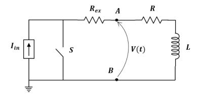
Figure 3-16: Circuit used to determine the value of the available inductors.
