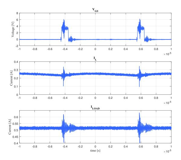
Figure 3-22: Wrong waveforms observed during buck tests.
