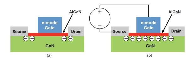
Figure 2-6: (a) An enhancement-mode (e-mode) device depletes the 2DEG with zero volts on the gate. (b) By applying a positive voltage to the gate, the electrons are attracted to the surface, re-establishing the 2DEG [27].
