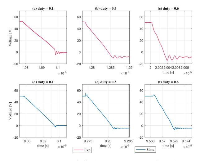
Figure 4-16: Drain-to-source  $(V_{DS})$  voltage transients produced in SW2 at the turnon for different duty-cycles at  $V_{in} = 50V$ : (a) Experimental at duty = 0.1; (b) Experimental at duty = 0.3; (c) Experimental at duty = 0.6; (d) Simulation at duty = 0.1; (e) Simulation at duty = 0.3; (f) Simulation at duty = 0.6.
