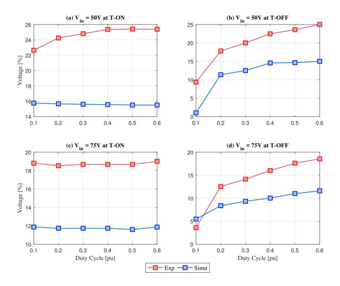
Figure 4-17: Drain-to-source  $(V_{DS})$  peak voltages produced in switch 1 (SW1) at the turn-on and turon-off events for different duty-cycles and different test voltages: (a) turn-on at  $V_{in} = 50V$ ; (b) turn-off at  $V_{in} = 50V$ ; (c) turn-on at  $V_{in} = 75V$ ; (d) turn-off at  $V_{in} = 75V$ .
