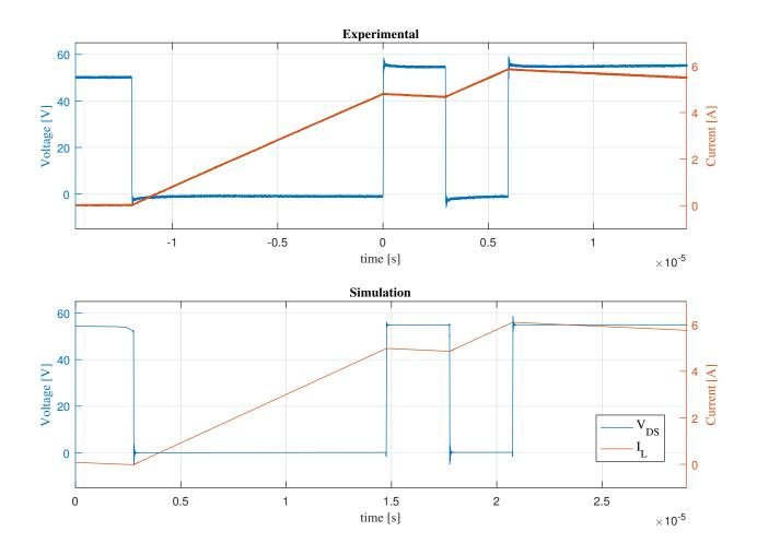
Figure 4-1: Drain-to-source voltage and inductor current observed in the DPT for  $V_{in} = 50V$  and I = 5A.
