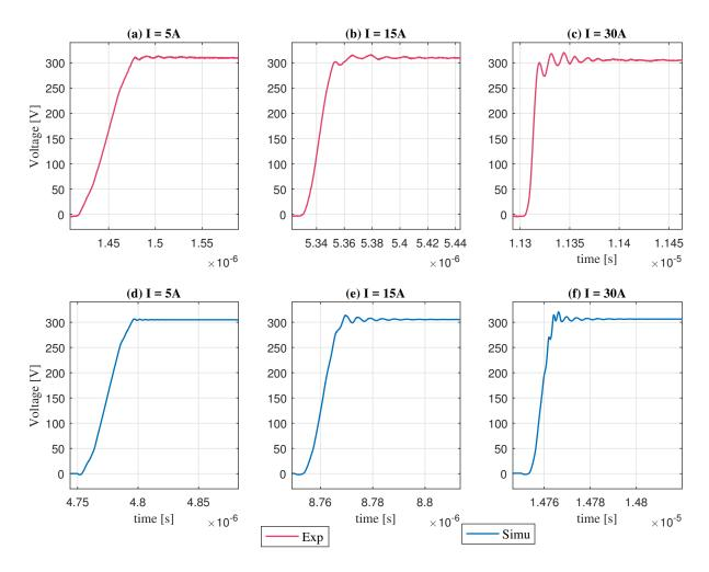
Figure 4-4: Drain-to-source  $(V_{DS})$  voltage transients produced at the turn-off for different current levels at  $V_{in} = 300V$ : (a) Experimental at 5A; (b) Experimental at 15A;(c) Experimental at 30A;(d) Simulation at 5A;(e) Simulation at 15A;(f) Simulation at 30A.
