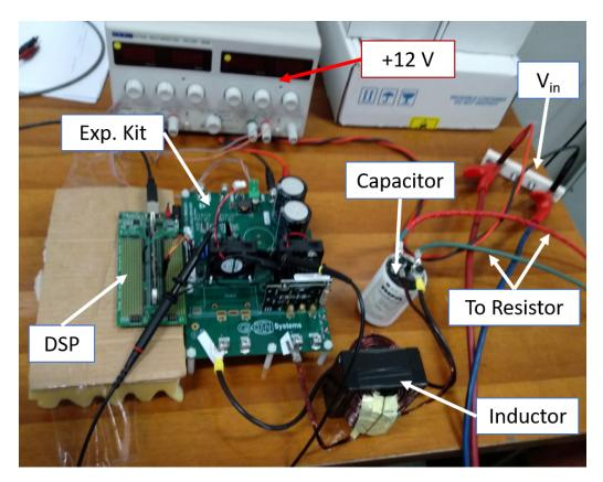
Figure 3-23: Physical assembly used for the buck converter.
