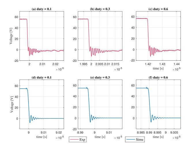
Figure 4-14: Drain-to-source  $(V_{DS})$  voltage transients produced in SW1 at the turnon for different duty-cycles at  $V_{in} = 50V$ : (a) Experimental at duty = 0.1; (b) Experimental at duty = 0.3;(c) Experimental at duty = 0.6;(d) Simulation at duty = 0.1;(e) Simulation at duty = 0.3;(f) Simulation at duty = 0.6.
