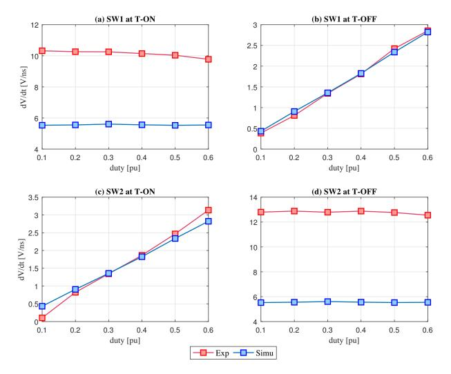
Figure 4-20: Drain-to-source  $(V_{DS}) dV/dt$  in [V/ns] produced in switch 1 (SW1) and switch 2 (SW2), at turn-on and turn-off events for  $V_{in} = 75V$  at different duty-cles: (a) SW1 and turn-on; (b) SW1 and turn-off;(c) SW2 and turn-on;(d) SW2 and turnoff.
