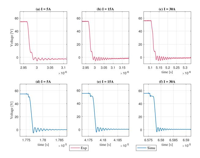
Figure 4-5: Drain-to-source  $(V_{DS})$  voltage transients produced at the turn-on for different current levels at  $V_{in} = 50V$ : (a) Experimental at 5A; (b) Experimental at 15A;(c) Experimental at 30A;(d) Simulation at 5A;(e) Simulation at 15A;(f) Simulation at 30A.
