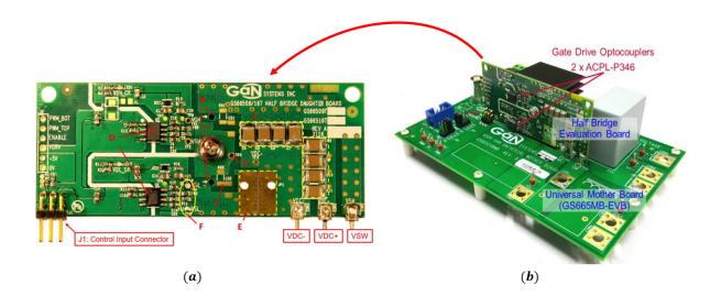
Figure 3-3: (a) GS66508T/GS66516T-EVBDB GaN E-HEMT top side daughter board 650V. (b) GS665MB-EVB Evaluation Platform.
