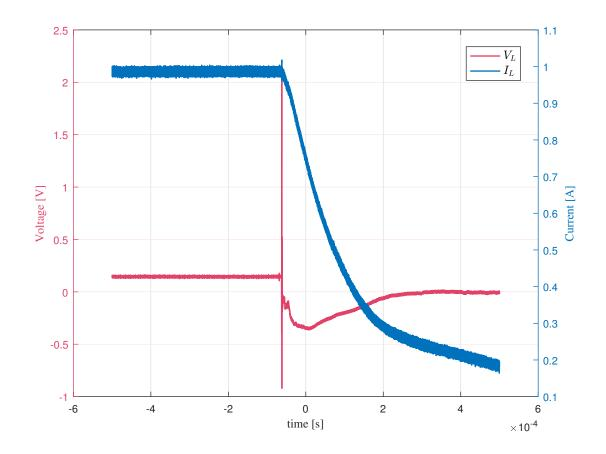
Figure 3-18: Inductor current and voltage signals obtained during the test performed to get the inductance value.
