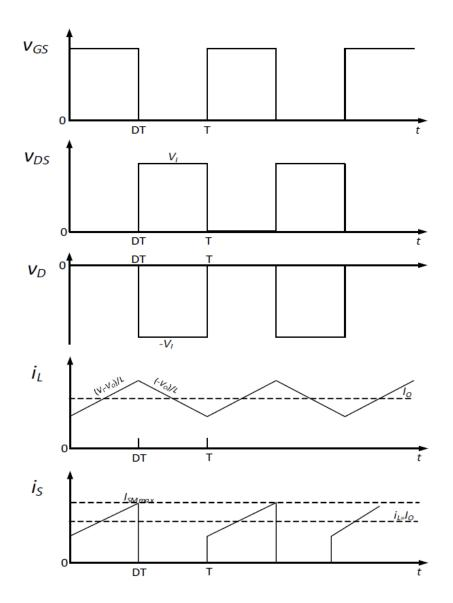
Figure 3-15: Buck switching waveforms corresponding to the two possible states when operating in CCM.
