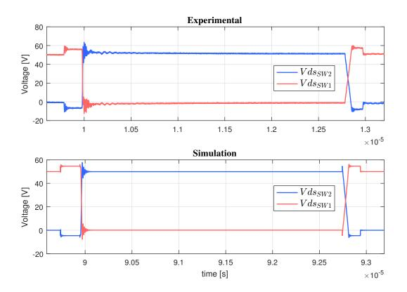
Figure 4-12: Drain-to-source  $(V_{DS})$  voltage transients produced at the turn-on and turn-off events in the synchronous buck converter in the experimental and simulation results.
