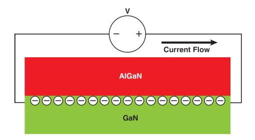
Figure 2-4: By applying a voltage to the 2DEG an electric current is induced in the crystal [27].
