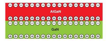
Figure 2-3: Simplified cross section of a GaN/AlGaN heterostructure showing the formation of a 2DEG due to the strain-induced polarization at the interface between the two materials [27].
