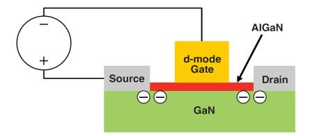
Figure 2-5: By applying a negative voltage to the gate of the device, the electrons in the 2DEG are depleted out of the device. This type of device is called a depletion-mode (d-mode) HEMT [27].
