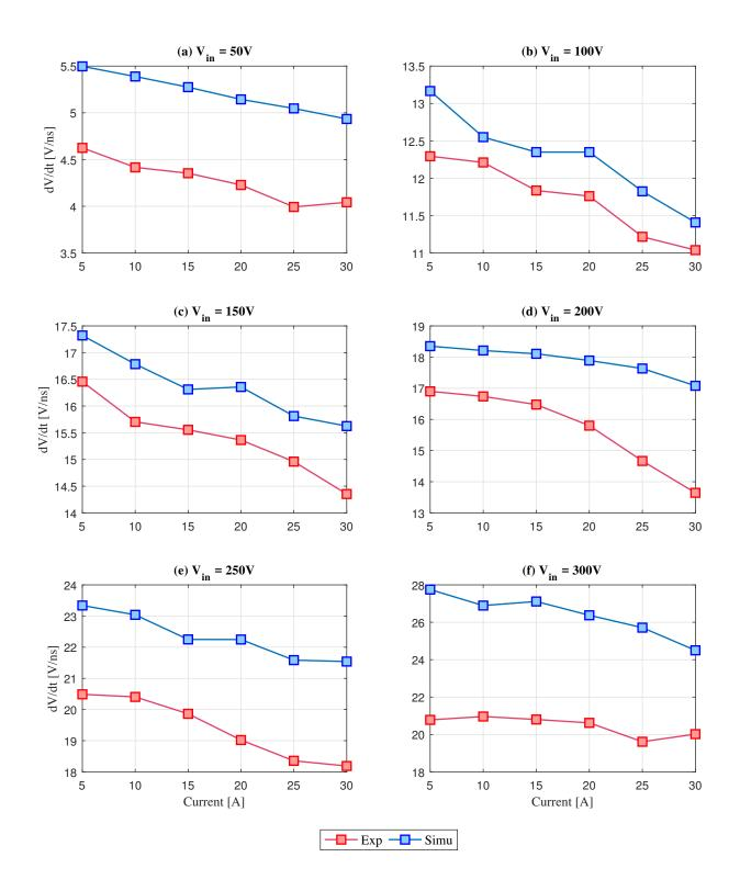
Figure 4-11: Drain-to-source  $(V_{DS}) dV/dt$  in [V/ns] produced at the turn-on event for different current levels and different test voltages: (a)  $V_{in} = 50V$ ; (b)  $V_{in} = 50V$ ;(c)  $V_{in} = 50V$ ;(d)  $V_{in} = 50V$ ;(e)  $V_{in} = 50V$ ;(f)  $V_{in} = 50V$ .
