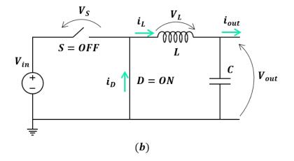
Figure 3-14: Equivalent circuit of the buck converter when operating in CCM: (a) Switch = ON and Diode = OFF; (b) Switch = OFF and Diode = ON.
