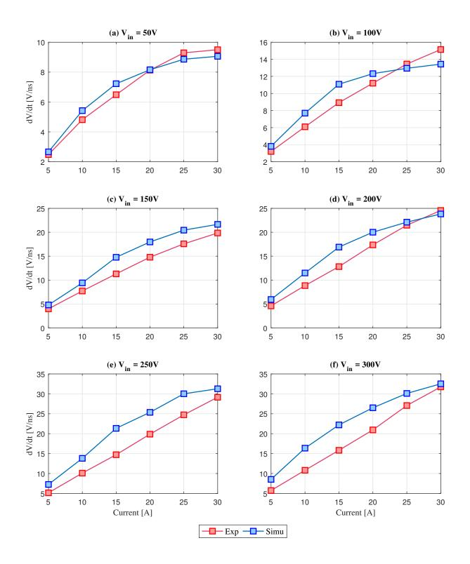
Figure 4-10: Drain-to-source  $(V_{DS}) dV/dt$  in [V/ns] produced at the turn-off event for different current levels and different test voltages: (a)  $V_{in} = 50V$ ; (b)  $V_{in} = 50V$ ;(c)  $V_{in} = 50V$ ;(d)  $V_{in} = 50V$ ;(e)  $V_{in} = 50V$ ;(f)  $V_{in} = 50V$ .
