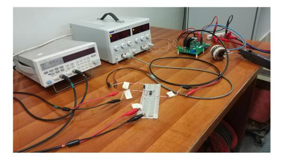
Figure 3-4: First assembly used to perform the double-pulse test.
