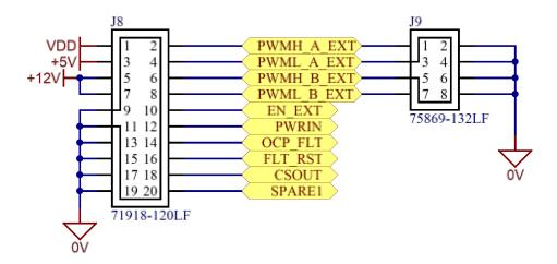
Figure 3-8: Pin connectors used to transmit the pulse signals to the gate drivers of the GaN HEMTs from the motherboard to the IMS.
