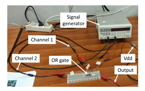
Figure 3-10: Assembly used to create the required double pulses to perform the double-pulse test with the signal generator and the OR gate.
