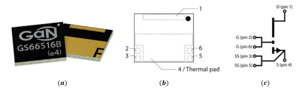
Figure 3-9: (a) SMD package for the used GaN HEMTs. (b) Terminals of the used GaN HEMTs in relation with (c), which shows the electrical symbol representation of the transistor.
