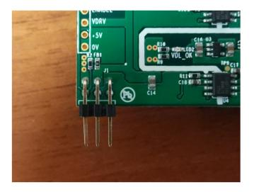
Figure 3-5: Poor pin connectors used to transmit the control signals from the mother board (connected with the pulse source generator) to the daugther board.
