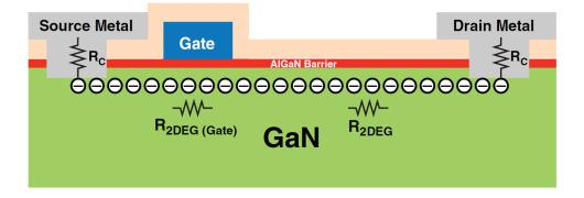
Figure 2-9: Cross section of a GaN HEMT, showing the major components of  $R_{DS(on)}$  [27].
