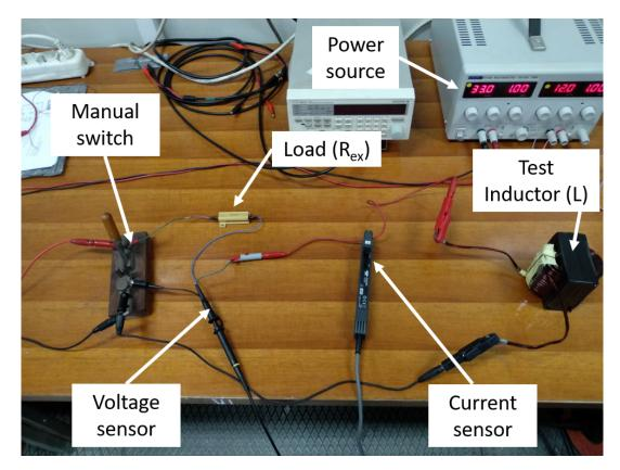
Figure 3-17: Real circuit used to determine the value of the available inductors.
