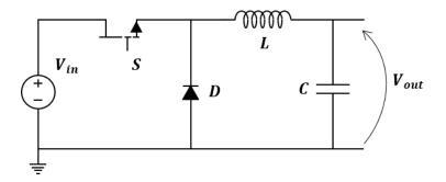
Figure 3-13: Electrical scheme of the buck converter.
