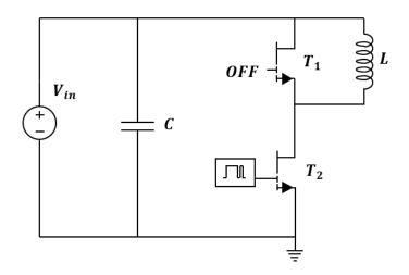
Figure 3-1: Double-pulse test circuit - Inductive load.
