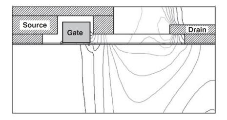
Figure 2-8: The device in Figure 2.6 showing the electric fields when voltage is applied from drain to source.
