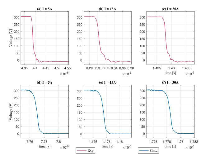
Figure 4-7: Drain-to-source  $(V_{DS})$  voltage transients produced at the turn-on for different current levels at  $V_{in} = 300V$ : (a) Experimental at 5A; (b) Experimental at 15A;(c) Experimental at 30A;(d) Simulation at 5A;(e) Simulation at 15A;(f) Simulation at 30A.
