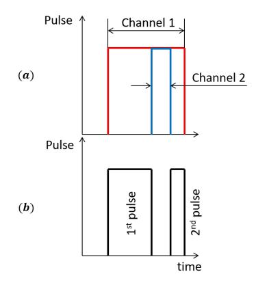
Figure 3-11: (a) Commands produced by the generator source channels. (b) Pulses produced by combining the signal generator commands and the OR gate.
