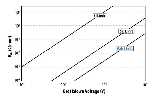
Figure 2-1: Theoretical on-resistance vs blocking voltage capability for silicon, siliconcarbide, and gallium nitride [3].
