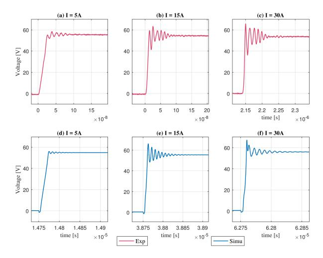
Figure 4-2: Drain-to-source  $(V_{DS})$  voltage transients produced at the turn-off for different current levels at  $V_{in} = 50V$ : (a) Experimental at 5A; (b) Experimental at 15A;(c) Experimental at 30A;(d) Simulation at 5A;(e) Simulation at 15A;(f) Simulation at 30A.
