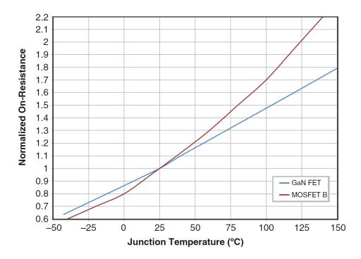
Figure 2-10: Normalized  $R_{DS_{ON}}$  vs. temperature for a 100V enhancement-mode GaN transistor (EPC2010) compared with an Si power MOSFET with similar ratings [39].
