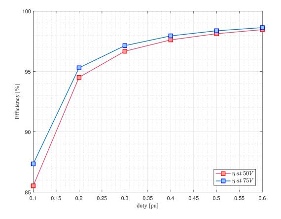
Figure 4-21: Efficiency of the synchornous buck converter obtained in the simulations for different input voltage levels at different duty cycles.
