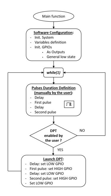
Figure 3-12: Flow chart of the program created to generate the pulses for the doublepulse test.
