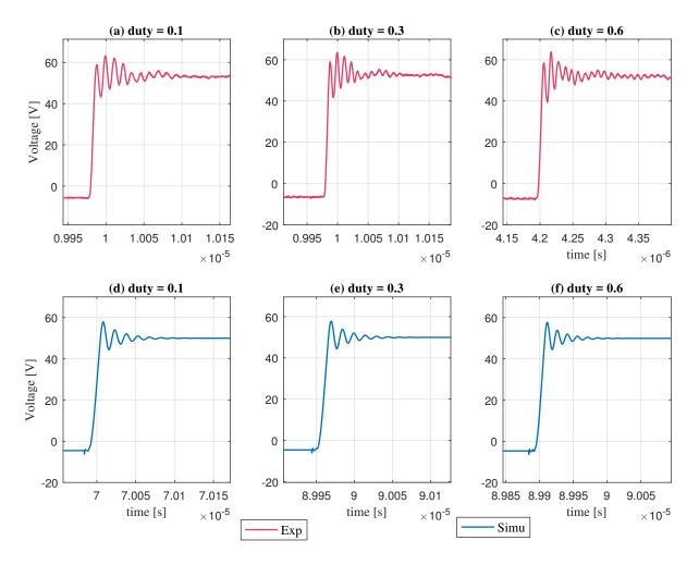
Figure 4-15: Drain-to-source  $(V_{DS})$  voltage transients produced in SW2 at the turnoff for different duty-cycles at  $V_{in} = 50V$ : (a) Experimental at duty = 0.1; (b) Experimental at duty = 0.3; (c) Experimental at duty = 0.6; (d) Simulation at duty = 0.1; (e) Simulation at duty = 0.3; (f) Simulation at duty = 0.6.
