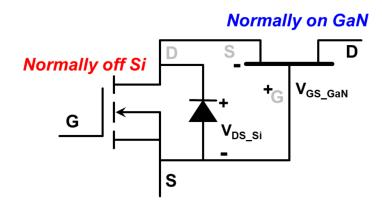
Figure 2-7: Cascode configuration combining a high voltage normally on GaN HEMT with a low voltage normally off silicon MOSFET.
