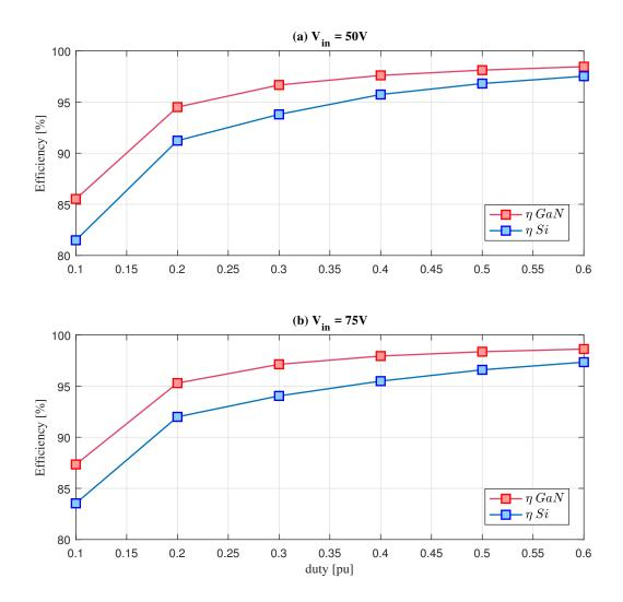
Figure 4-22: Comparison of the synchornous buck converter efficiency obtained in the simulations when using GaN and Si technology for different input voltage levels at different duty cycles.
