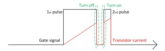
Figure 3-2: Double-pulse test signals - Inductive load.
