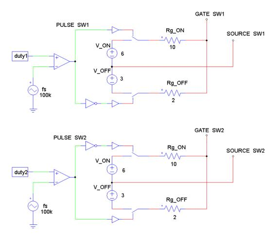
Figure 3-20: Gate drive circuit used to create the gate drive signals to control the buck converter.
