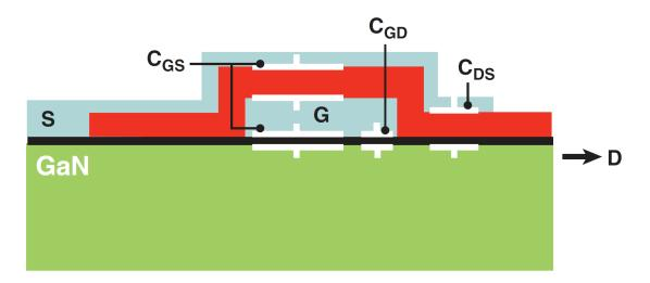
Figure 2-11: Schematic of GaN transistor capacitive sources [27].
