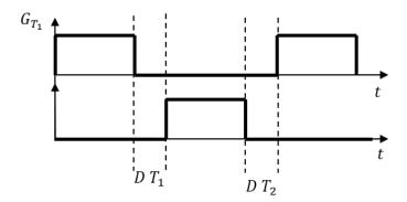
Figure 3-19: Deadtimes  $DT_1$  and  $DT_2$  are inserted between the gating signals.
