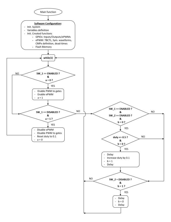
Figure 3-24: Flow chart of the program created to generate the pulses for the buck test.
