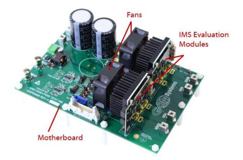
Figure 3-6: Experimental Evaluation Kit: GSP65RxxHB evaluation motherboard and 650V high power insulated metal substrate (IMS) evaluation modules.
