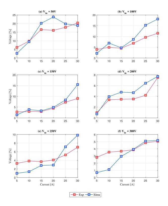
Figure 4-8: Drain-to-source  $(V_{DS})$  peak voltages produced at the turn-off overshoot for different current levels and different test voltages: (a)  $V_{in} = 50V$ ; (b)  $V_{in} = 50V$ ;(c)  $V_{in} = 50V$ ;(d)  $V_{in} = 50V$ ;(e)  $V_{in} = 50V$ ;(f)  $V_{in} = 50V$ .
