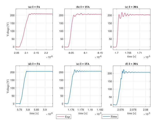
Figure 4-3: Drain-to-source  $(V_{DS})$  voltage transients produced at the turn-off for different current levels at  $V_{in} = 200V$ : (a) Experimental at 5A; (b) Experimental at 15A;(c) Experimental at 30A;(d) Simulation at 5A;(e) Simulation at 15A;(f) Simulation at 30A.
