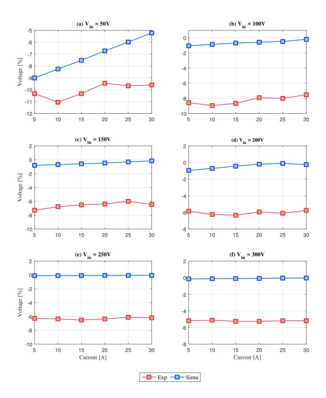
Figure 4-9: Drain-to-source  $(V_{DS})$  peak voltages produced at the turn-on overshoot for different current levels and different test voltages: (a)  $V_{in} = 50V$ ; (b)  $V_{in} = 50V$ ;(c)  $V_{in} = 50V$ ;(d)  $V_{in} = 50V$ ;(e)  $V_{in} = 50V$ ;(f)  $V_{in} = 50V$ .
