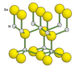
Figure 2-2: Schematic of wurtzite GaN [27].
