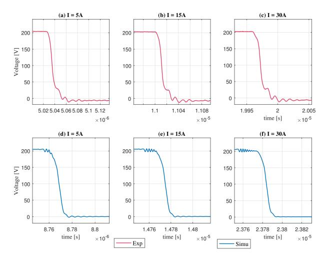
Figure 4-6: Drain-to-source  $(V_{DS})$  voltage transients produced at the turn-on for different current levels at  $V_{in} = 200V$ : (a) Experimental at 5A; (b) Experimental at 15A;(c) Experimental at 30A;(d) Simulation at 5A;(e) Simulation at 15A;(f) Simulation at 30A.
