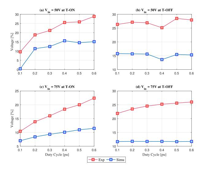
Figure 4-18: Drain-to-source  $(V_{DS})$  peak voltages produced in switch 2 (SW2) at the turn-on and turon-off events for different duty-cycles and different test voltages: (a) turn-on at  $V_{in} = 50V$ ; (b) turn-off at  $V_{in} = 50V$ ; (c) turn-on at  $V_{in} = 75V$ ; (d) turn-off at  $V_{in} = 75V$ .
