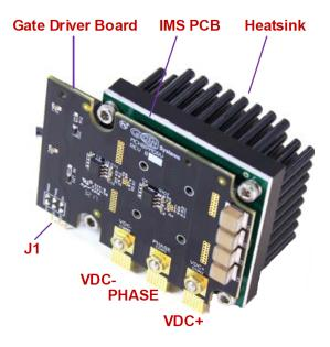
Figure 3-7: Insulated metal substrate (IMS) evaluation module used in the motherboard.
