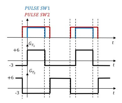
Figure 3-21: Gate drive signals used to control the synchronous-buck converter.
