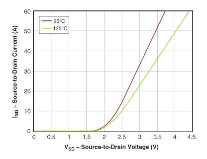
Figure 2-12: Body-diode forward drop vs. source-drain current and temperature by EPC2010 [39].
