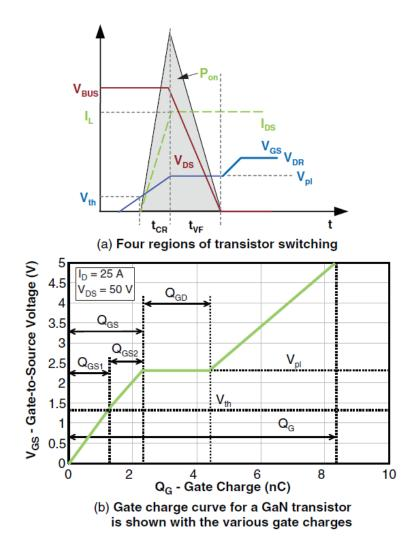
Figure 2-13: Gate charge vs. gate voltage showing different gate charge components for an EPC2010 GaN transistor [39].
