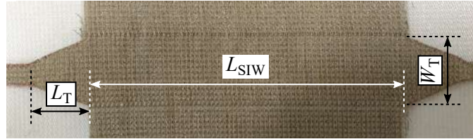
Figure 3.27: Top view of the manufactured back to back microstrip to TIW transition.
