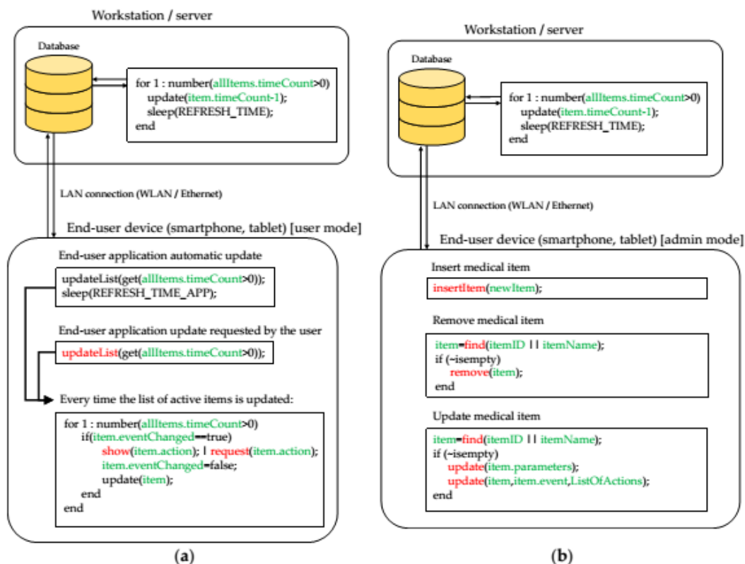
Figure 5. (a) Pseudo-code showing the interaction between an end-user and the information stored in the database. (b) Pseudo-code illustrating how new items are introduced in the database when the user is authenticated as administrator. Information associated to the database is highlighted in green, while end-user actions using the mobile application are denoted in red.
