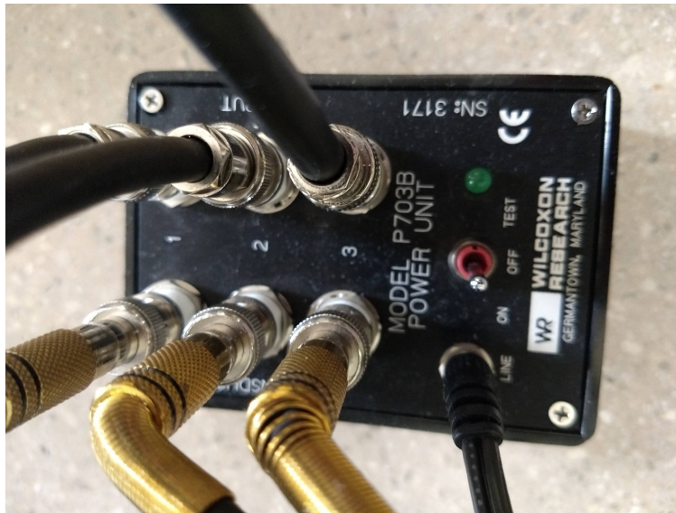
Figure 2.11: Wilcoxon Research power unit for accelerometers.
