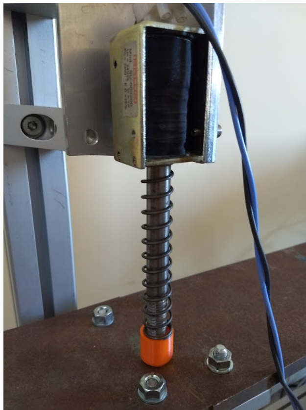
Figure 2.6: Hammer with its 3D-printed cover in orange.
