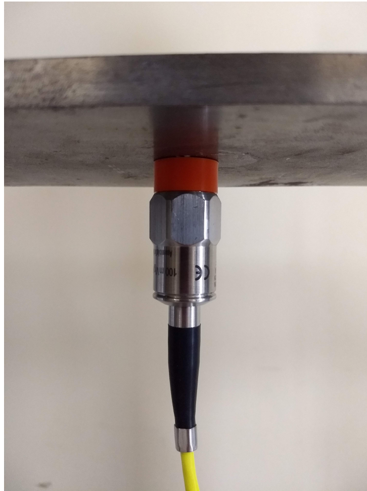
Figure 2.10: Wilcoxon Research accelerometer with its 3D-printed cover in orange.
