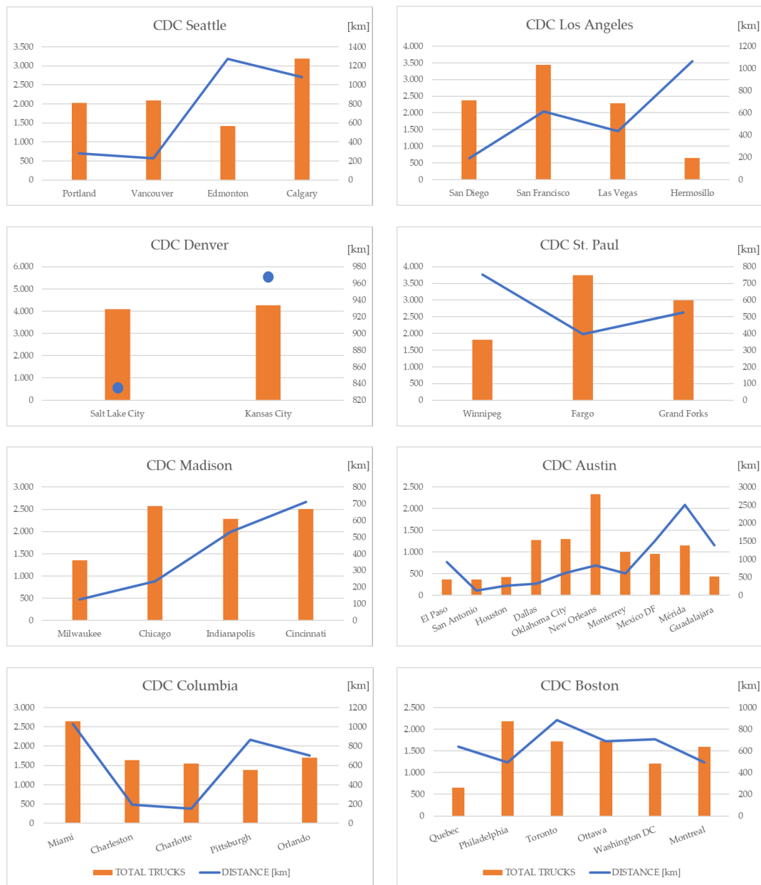
FIGURE 2.18: Total number of trucks needed in a year and route distance between all 8 CDCs in United States and their respective RDCs.
