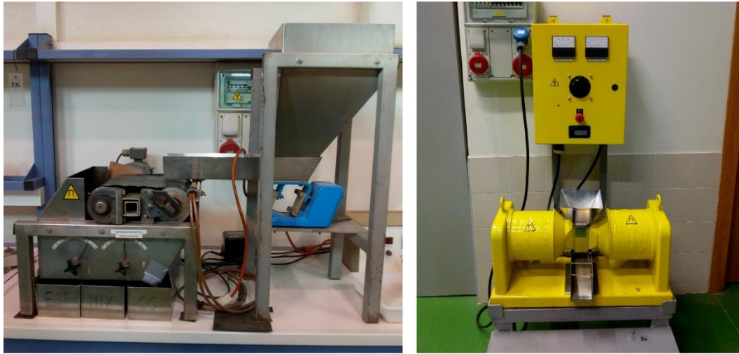
Figure 1.6 Left.- Dry-HIMS Model L/P 10:30 of International Process Systems Inc. (U.S. PATENT) Right.- Wet-HIMS Model OUTOTEC Laboratory 3X4L
