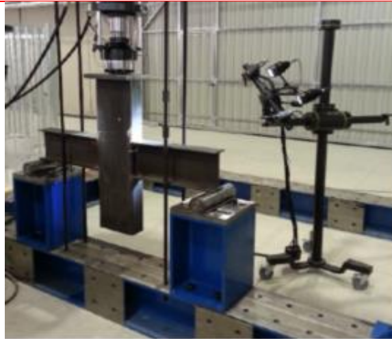
Fig. 3 Test rig with Aramis DIC system
