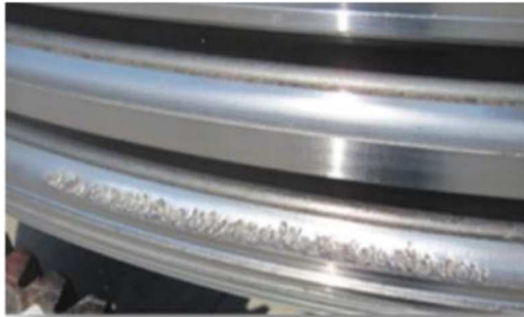
Figure 1. Example of the RCF damage in a pitch bearing [9].
