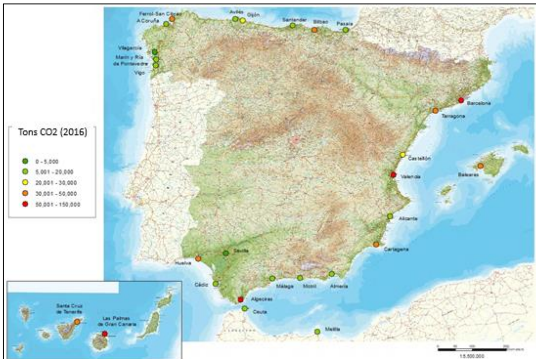
Figure 2. Potential reductions in CO2 emissions by Port Authority if on-shore power supply were used
