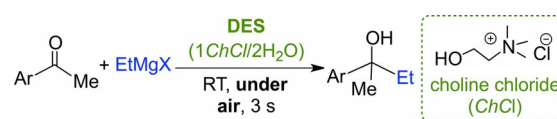
Scheme 1. Addition of RMgX reagents to ketones under air at ambient temperature by using ChCl-based DESs. [5a]
