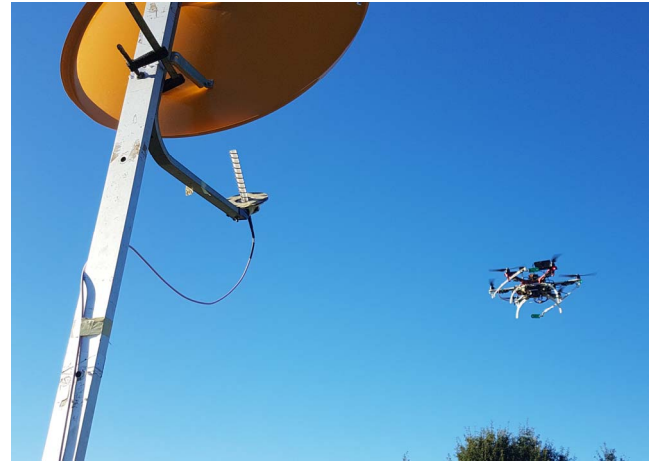
Fig. 5. Picture of the modified UASAM prototype for simultaneous acquisition of the NF at two surfaces, when measuring the NF radiated by the offset reflector antenna.
