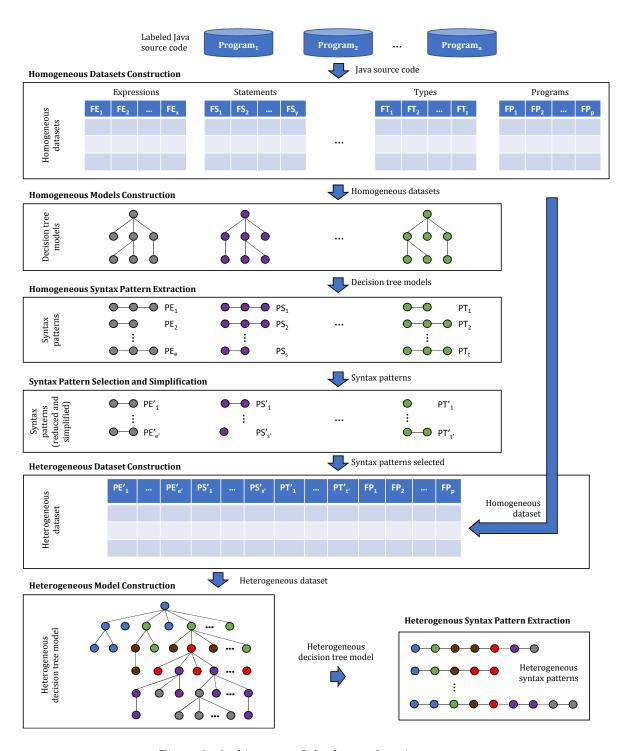
Figure 2: Architecture of the feature learning process.
