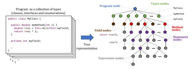
Figure 1: Program representation as heterogeneous compound syntax trees.
