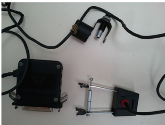
Fig. 3. Extensometer used to obtain Young's modulus.
