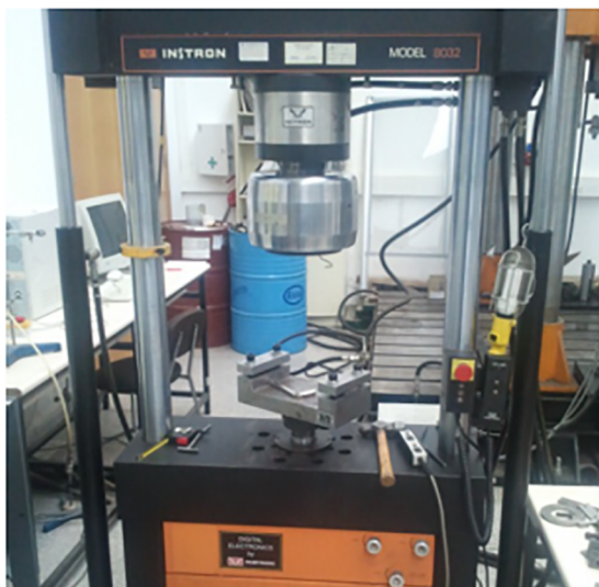
Fig. 1. Universal testing machine used for tensile tests.
