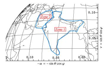
Fig. 3. Footprint of the southern Asian coverage, with (u,v) coordinates in the satellite coordinate system.
