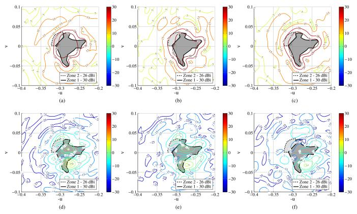
Fig. 4. Copolar (top) and crosspolar (bottom) radiation patterns for Y polarization (all of them in dBi) at 13.20 GHz for (a), (d) stage 1; (b), (e) stage 2; and (c), (f) stage 3 of the broadband design procedure.
